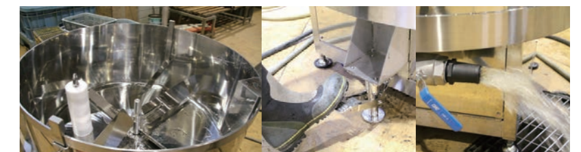
Inside the mixing tank Easy dehydrating by using foot pedal
