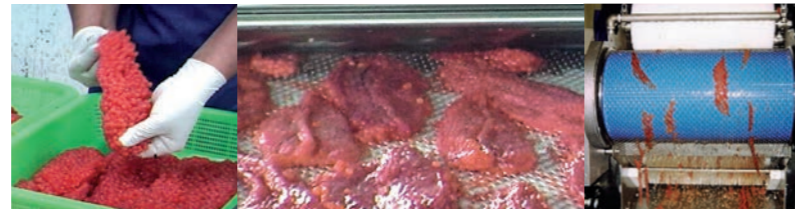
Preparation Split open at center of eggs. Feeding to conveyor Feeding eggs as face "open part" down to conveyor. After that the machine will separate eggs from skin automatically. Discharging skin
