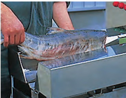
Continuous insertion (Fish Back on the top Fish Belly on the bottom)
